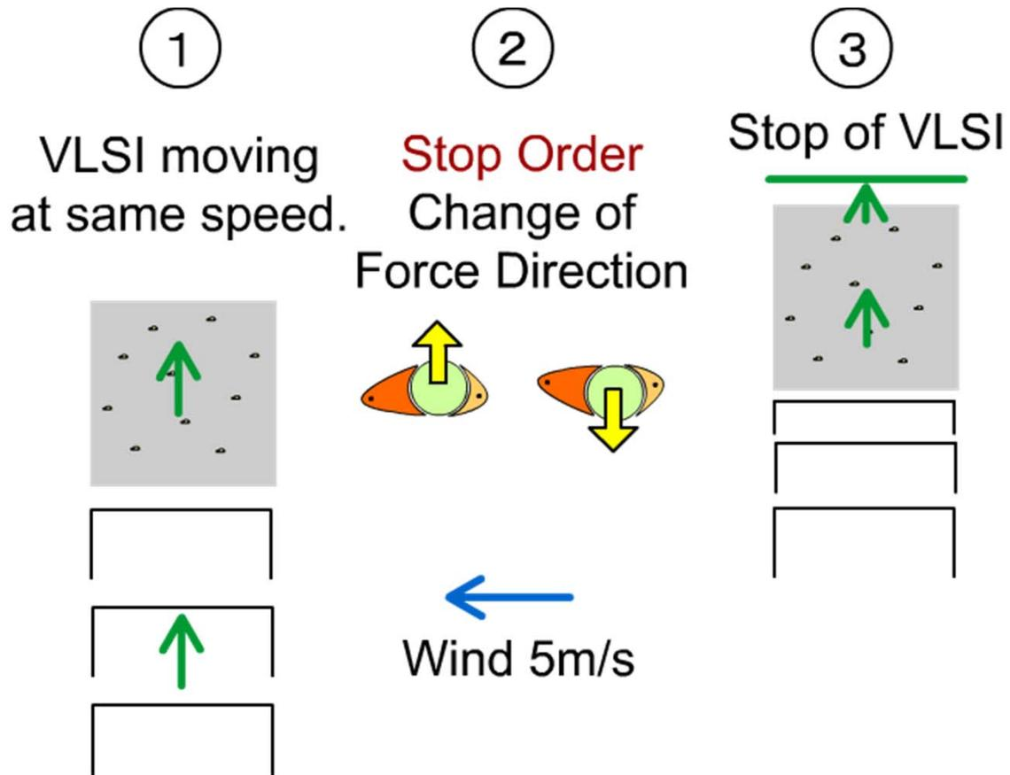
If we can make the wind force which we got by "Outline examination(1)" to stop, it will be 390000 kg.m/s<sup>2</sup> with 10 Lift Force Generators.
